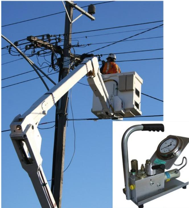
*A small and mobile Power Pack increases the tool options when working far from the engine.*
